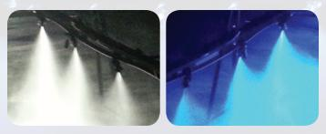
An accurate and proper sprayer boom illumination will enable you to see and monitor the nozzles and spray pattern from the cab.
